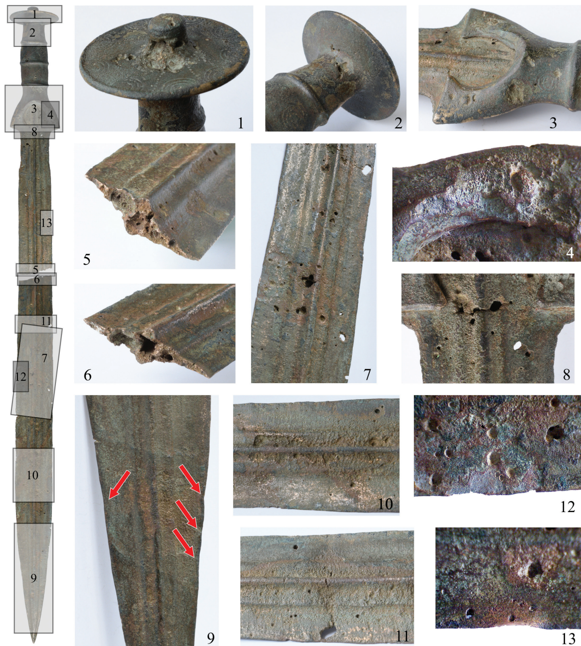
Fig. 7. Macroscopic observation of the sword with casting faults and recent deterioration marks: 1. casting fault at the base of the knob; 2. casting fault under the pommel disc; 3–4. casting faults on the shoulders and around the rivet; 5–6. porosity visible in cross-section; 7–8. gas-porosity traces on the surface of the blade; 9. incomplete filling; 10. corroded-like surface due to porosity; 11. recent crack across the blade; 12–13. recent chipped cutting edge.
